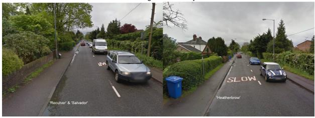
There is potential scope for a raised junction table at the junction with Springfield Park, (below left). There are inspection covers to services in the main carriageway and a surface water drain in the centre of the junction that would require additional works to address. Again this location does have the benefit of being directly under a street light for improved nightime visibility.
